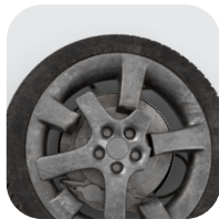
Tyre & Rim Damage
